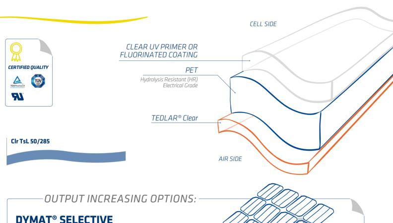
Optional white grid incorporated in the backsheet that turns the space in between the cells and the borders into a highly reflective area for significant output improvement. The grid layout is defined according to customer's cell shape and size.
